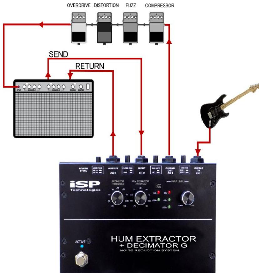
Channel 2 can be inserted after the pedal chain if a series loop is not available in the setup.
