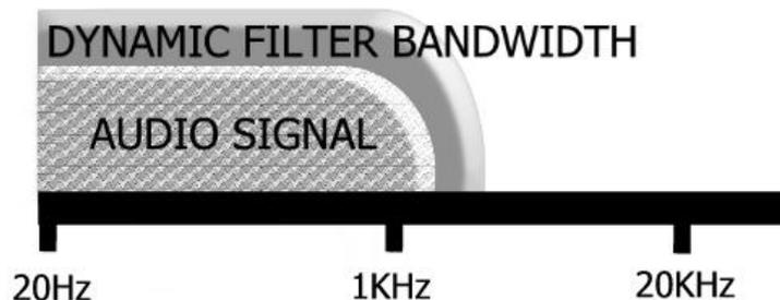
The release time of the dynamic filter is controlled by the Time Vector Processing circuit and our new patent pending DECIMATOR X technology, which determines the release characteristics of the input signal and automatically varies the release response of the dynamic filter.
