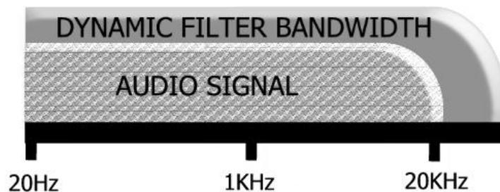
When the high frequency information in the input signal decreases the dynamic filter bandwidth will track the decrease in high frequency and eliminate high frequency noise that remains in the input signal. The simplified graph below shows the dynamic filter response when there is no high frequency audio above 1KHz.
