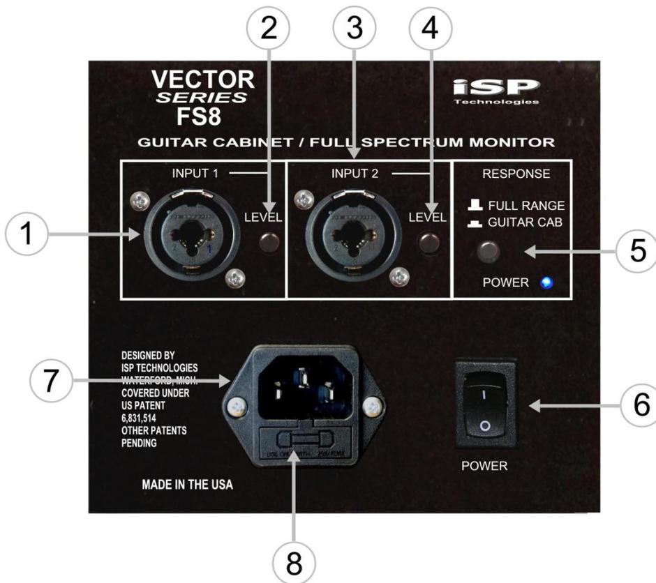
1. Channel 1 input / Combo Jack will accept either balanced XLR or ¼ inch plugs
