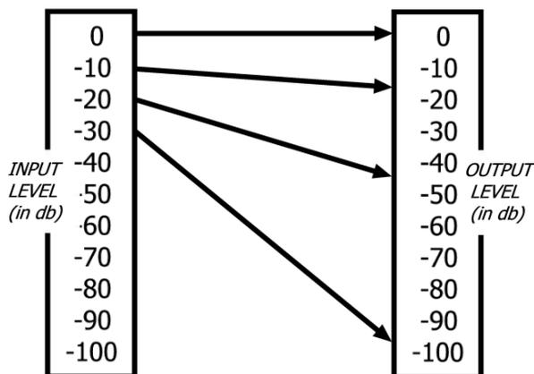
*As the input signal level decreases at the input below the threshold*
