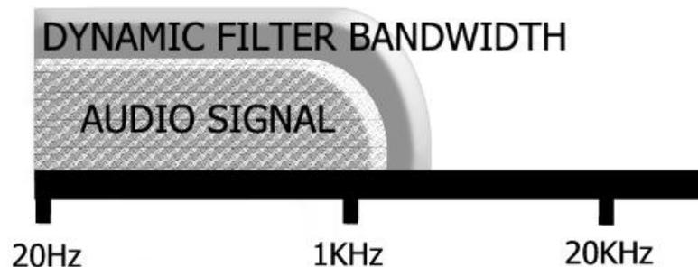
The release time of the dynamic filter is controlled by the Time Vector Processing circuit, which determines the release characteristics of the input signal and automatically varies the release response of the dynamic filter.
