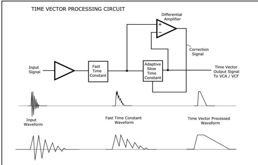
based on the difference between the fast time constant and the adaptive slow time constant to vary the release time to match the actual envelope of the input signal. Over a short period of time, the output signal will adjust to match the actual envelope of the input signal being played.
