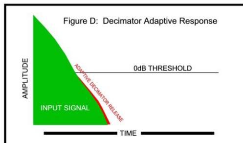
The figures to the left show the response difference that you get with a fixed release expander type noise gate vs. the Adaptive release response of the Decimator. Figure A and Figure B both
