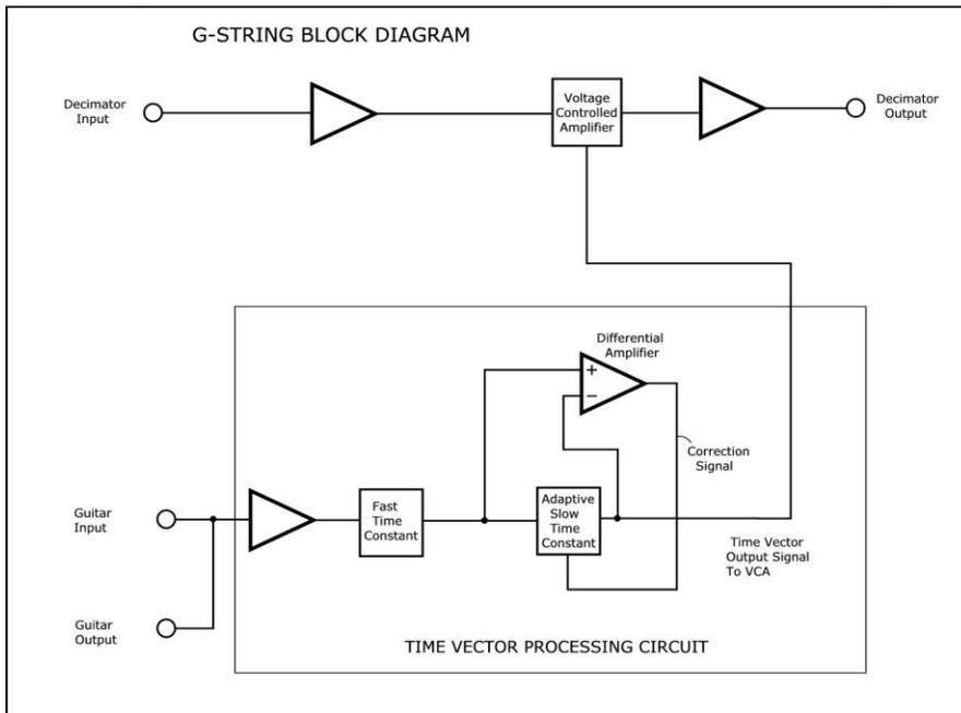
direct output of the guitar signal and also provide a block of Decimator noise reduction that can be inserted at the end of a chain of pedals or in the loop of a series effects loop. In this configuration you can switch between an extremely high gain signal and clean signal and everything in between and never need to adjust the threshold of the Decimator G-String. You can see in the simplified block
